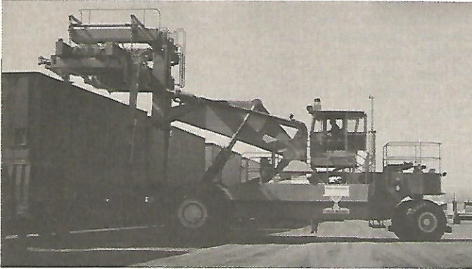
THE PIGGY PACKER is positioned for "lift-off."
