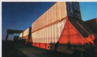
To improve service for intermodal shippers, Southern Pacific designed new cars that carry containers stacked two high. These open cars increase train capacity, reduce weight, and produce substantial savings in fuel.
