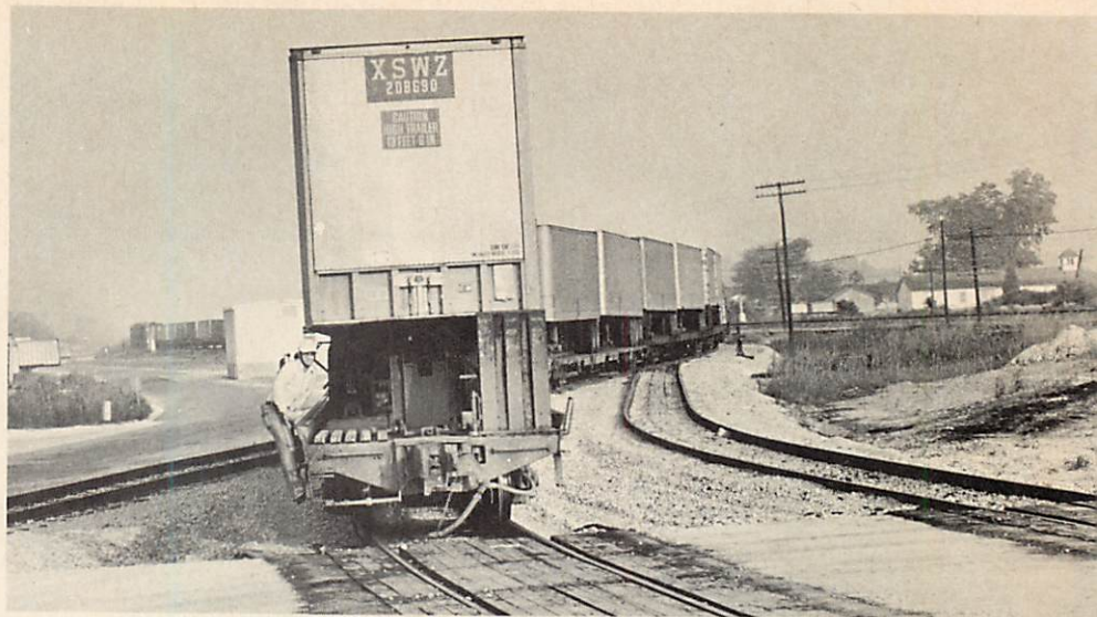
Cars loaded with containers and trailers are switched into one of New Orleans center's two new intermodal tracks, where they will be unloaded by straddle crane. Switchman R. Devellier, riding lead car, prepares to signal engineer. Portion of new office building and gate house is shown at left of train.
